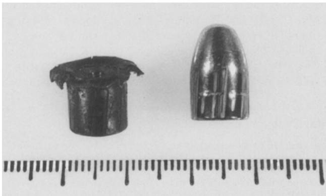
Fig. 1 The 2 types of 9 mm bullets used after recovery from the bullet collector. On the left, there is an Action-1 bullet after perforation of a hind leg. The firearm used was a H + K MP 5 submachine gun, impact velocity approximately 480 m/s. The cavity in the tip and the opening of the central channel can be seen. Part of the deformation zone has broken off. On the right, there is a FMJ bullet without deformation or fragmentation after perforation of a head. The pistol used was a SIG P210, impact velocity approximately 370 m/s. Contrary to the Action-1 bullet, the FMJ bullet does not show any prominent parts or cavities
